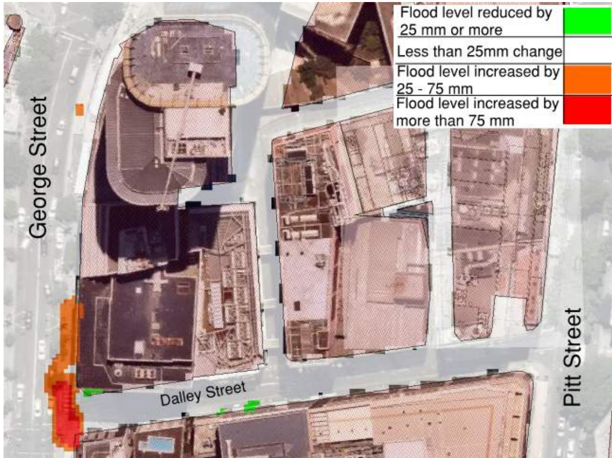
Figure 27 Impact of proposed threshold on flood levels: 5-year ARI
