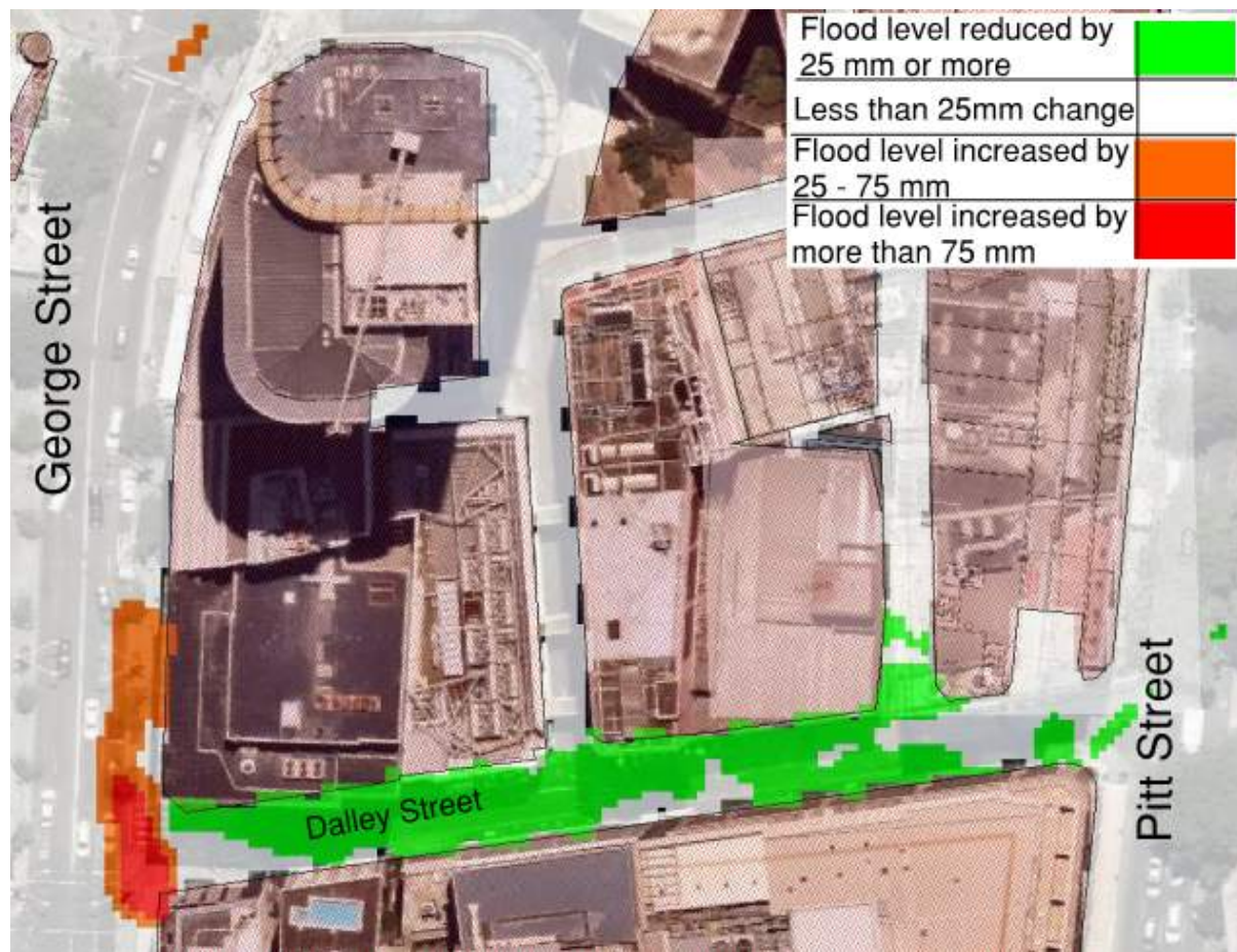
Figure 28 Impact of proposed threshold on flood levels: 100-year ARI
